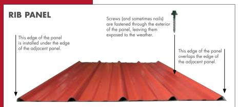
Ridges in the panel make it difficult to bend at the gutter edge of the roof to terminate cleanly and to provide protection against wind uplift. Foam is often used to fill the gaps between the panel and the deck. There are many different types of metal panels used by the construction industry. Each type of panel has its own application, depending on the type of building it's being installed on.
