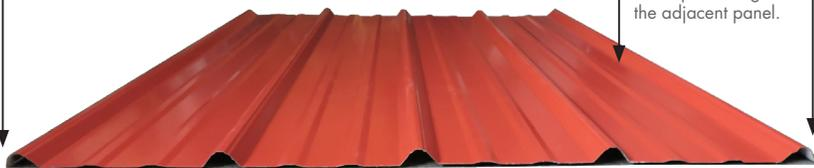
Ridges in the panel make it difficult to bend at the gutter edge of the roof to terminate cleanly and to provide protection against wind uplift. Foam is often used to fill the gaps between the panel and the deck.
